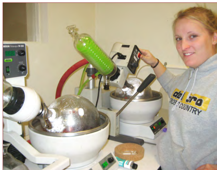
Trisha Buescher, a chemical engineer with Digital Solid State Propulsion, checking the Rotavapor instruments which reduce water content of one propellant ingredient. Photo courtesy of Judith Lancaster
